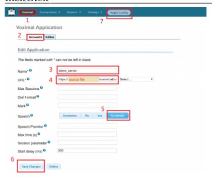
**5.** Set a call number to our account that just created, give it any number and name, the important part here is to set **destination**. it will be **voximal application** and link it to the account name that should appear on the list because we just made it \*\*(demo\_server)\*\*
